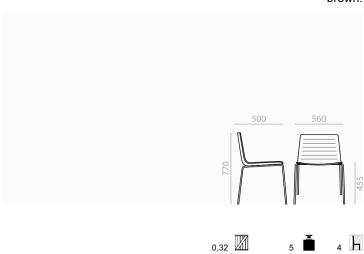
Frame 4-legged 18 mm. steel tube base with EPL-5 outdoor treatment. Polypropylene glides.
