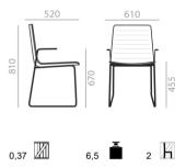
Frame Sled base of 12 mm diameter steel rod. Polypropylene glides.
